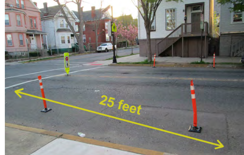
Parking should be prohibited within at least 25 feet of a crossing to ensure pedestrian visibility is not impeded.
