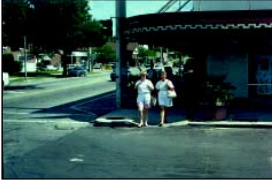
Figure 2.30: Two-foot corner on a traditional main street, Dade City, Florida.
