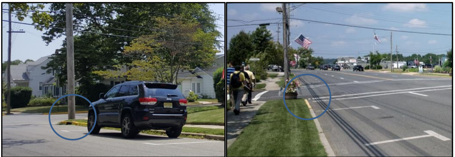
Fig. 7 and Fig. 8-Parking spaces too close to corner create pedestrian visibility risk
