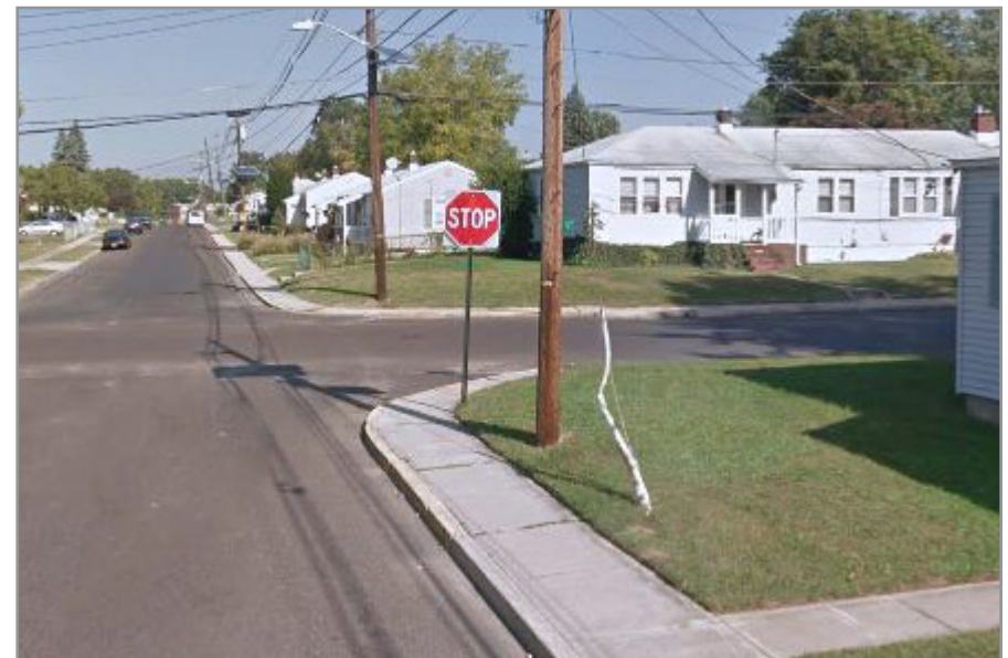
A utility pole properly located outside of the pedestrian right-of-way on Princeton Ave
