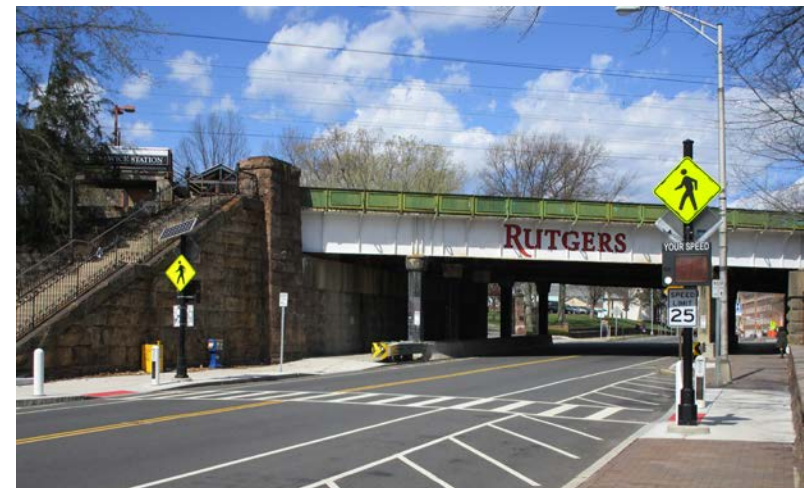
This crossing on George Street in New Brunswick demonstrates several features of high-visibility crosswalks, including street markings, reflective signage, speed limit signs, speed radars, and lighting.
