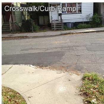
13 Misaligned intersection with ramps but no crosswalks or connections.
