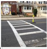
A mid-block crossing is provided however in lacks curb ramps or any advanced signage or signals.
