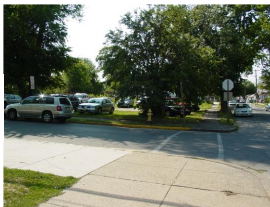
Front door access to Sharp's faculty parking lot has no curb ramps, no high visibility crosswalk
