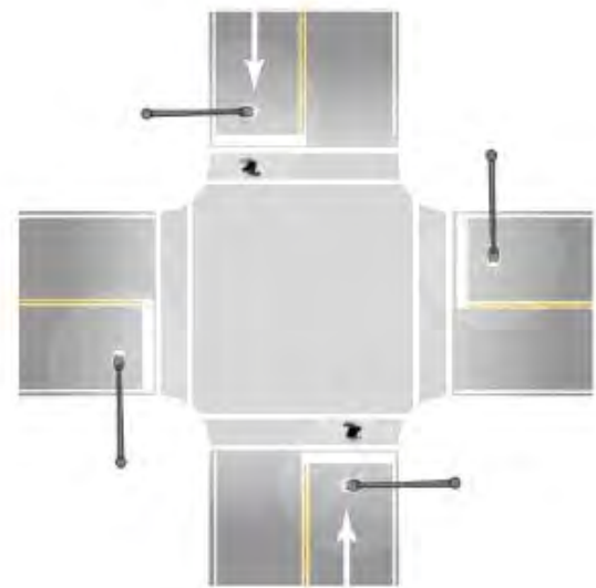
(Above) Traditional intersection lighting layout. (Below) New design for intersection lighting layout for crosswalks. Image: FHWA
