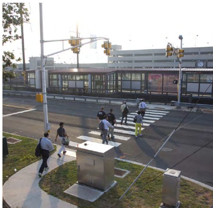
Pedestrian hybrid beacon provides improved pedestrian access across NJ 27 to Metropark rail station, where hundreds cross each day.
