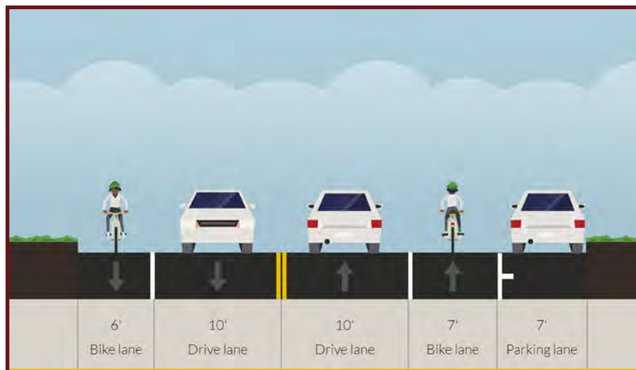
Figure 6: Potential Cross-Section to Accommodate Bike Lanes on Prospect Ridge Boulevard
