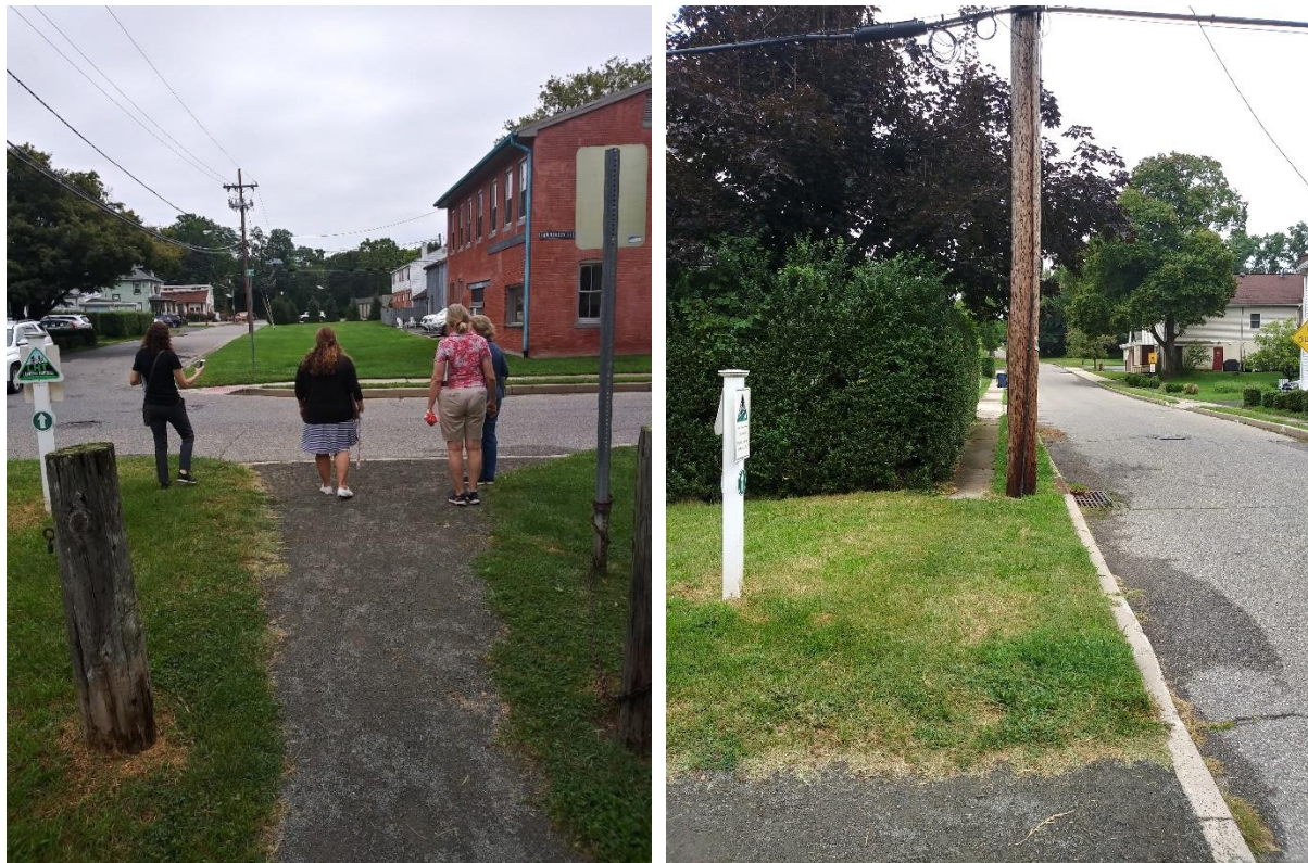
Figure 3 Johnson Trolley Line (JTL) ends on Phillips Avenue (left) without warning and opens into street without a marked crosswalk; the sidewalk access near the end of JTL is extremely narrow between a utility pole and overgrown hedges (right).
