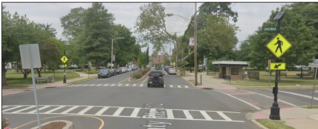
Picture 22: Example of a Rectangular Rapid Flashing Beacon (RRFB) used with pedestrian warning signs in Summit, NJ
