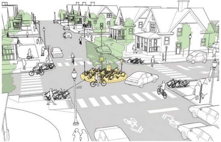
Picture 23: Illustration of a mini-roundabout. Source: National Association of City Transportation Officials (NACTO) Urban Street Design Guidelines
