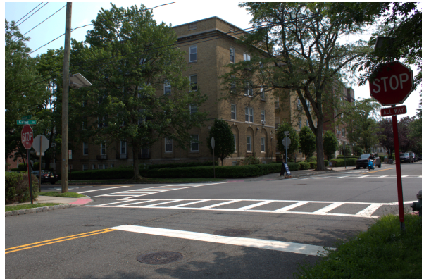
Stop All Way signs with high-visibility crosswalks and truncated dome pads. One stop sign on each side of Gates Ave. has a light-up feature and solar panels
