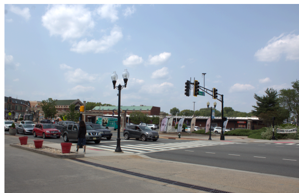
High-visibility crosswalk with pedestrian signals and a Pedestrian Signal button.
