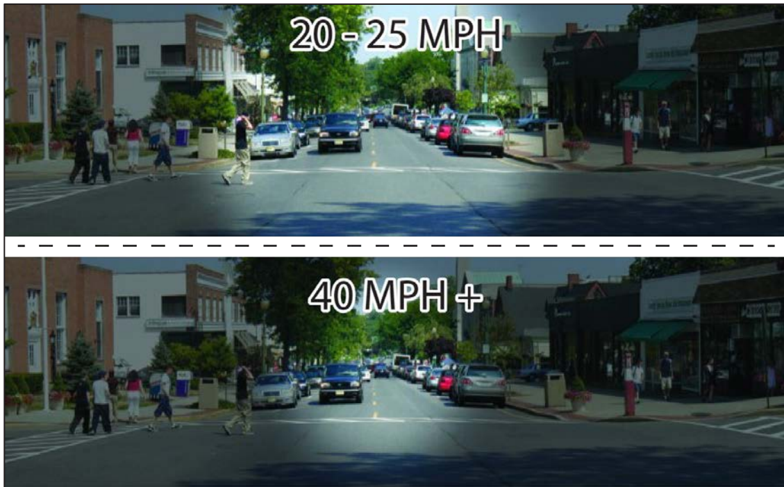
Effects of increased speed on a driver's visual focus (Source: NACTO)
